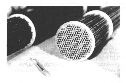
Figure 3: The CFRP cable type used for the Storchenbrücke (Stork Bridge) consists of 241 wires each with a diameter of 5 mm.
