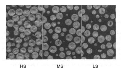
Figure 1b: . The load transfer media (LTM) is composed of aluminum oxide ceramic (Al<sub>2</sub>O<sub>3</sub>) granules with a typical diameter of 2 millimeters; HS=high stiffness, MS=medium stiffness, LS=low stiffness; right side=loadside
