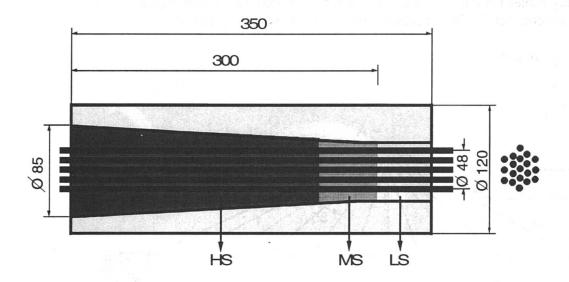
Figure 1a: Conical resin-cast termination; HS=high stiffness, MS=medium stiffness, LS=low stiffness; right side=loadside
