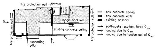
Figure 3: Bearing structure ground floor, after remodeling
