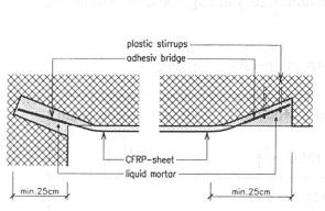
Figure 5: Anchorage of the CFRP-sheets in the concrete
