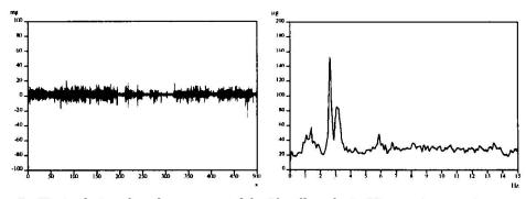
Figure 7: Typical signal and spectrum of the Nordbrücke in Vienna (composite structure)
