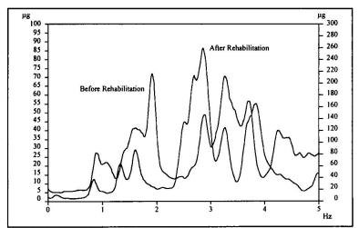
Figure 9: Comparison of spectra before during and after rehabilitaion
