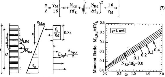
Fig. 3 Strain and stress distribution at in-plane flexural failure
