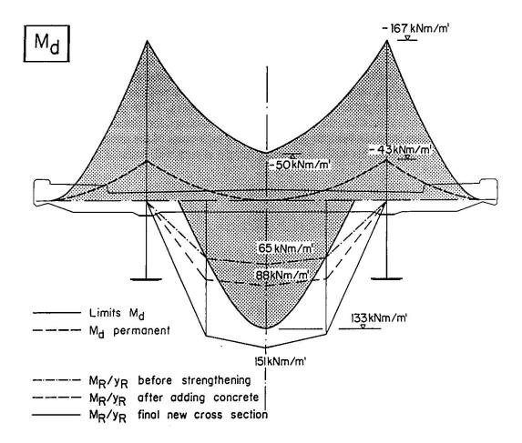
Fig 2. Transversal bending moment in bridge deck
