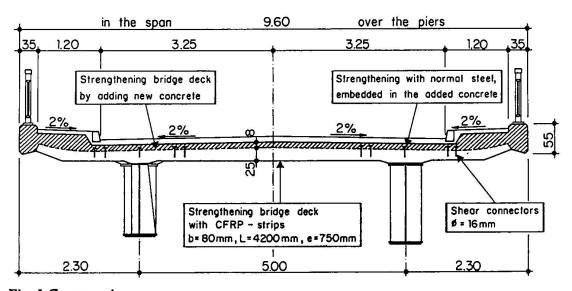
Fig. 1 Cross-section
