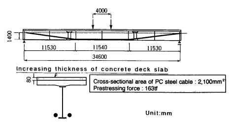
Fig. 5 Result of strengthening design by prestressing
