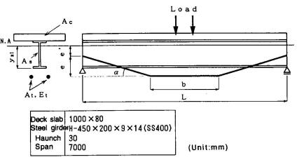
Fig. 3 Model symbols and section details used in parameter analysis
