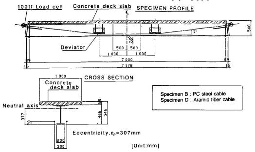
Fig. 2 Test specimen(for cables within the cross section)
