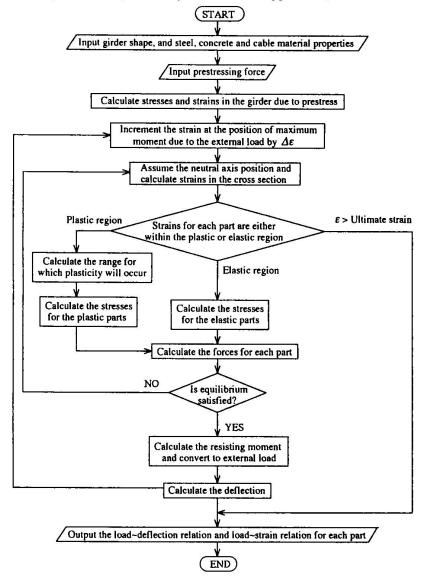
Fig. 1 Flowchart of incremental deformation method
