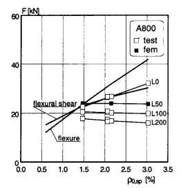
Fig. 4 Influence of reinforcement ratio  $\rho_{n.s.}$  on shear capacity as function of L
