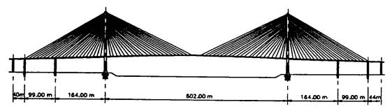
Fig. 5 YANGPU cable-stayed bridge in Shangai
