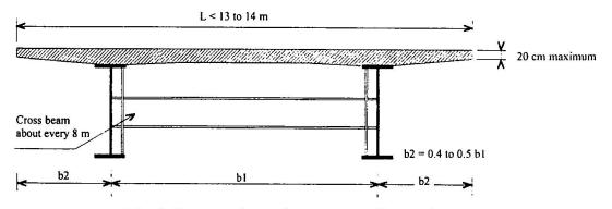
Fig. 1 Composite by-girder structure with cross beams
