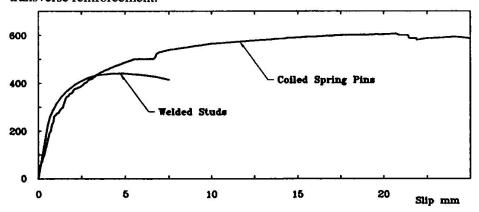
Figure 2 Typical Load-Slip Behaviour of Specimen Under Static Shear Loading
