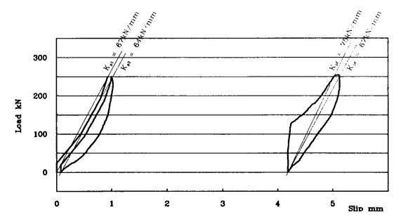
Figure 3 Typical Load-Slip Response in Specinien with 35mm Flanges
