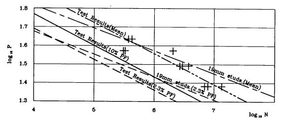
Figure 5 Load-Endurance Relationships for Coiled Spring Pin Connectors
