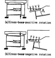
Fig.8 Behavior between slab and flange for cross-beam rotation
