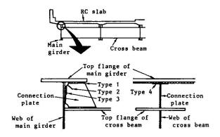
Fig.1 Fatigue cracks at cross-beam connections
