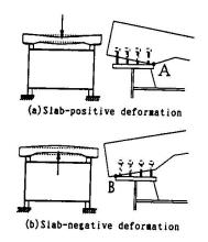
Fig. 7 Behavior between slab and flange for slab deformation
