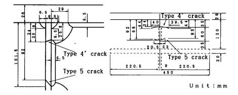
Fig. 6 Types 4' and 5 fatigue cracks at 5.1×10<sup>6</sup> cycles [Main girder B2-G1]
