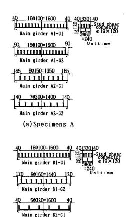
Fig.3 Stud arrangement
