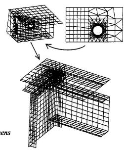
Fig. 10 Mesh division for specimens
