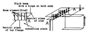
(a) Load-transfer-model for slab-positive deformation and cross-beam-positive rotation
