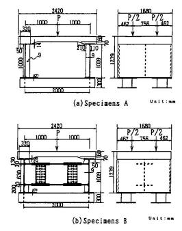
Fig. 2 Fatigue test specimens
