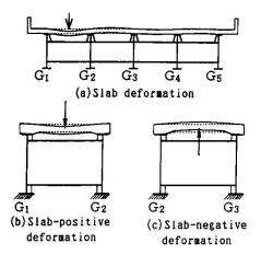
(a) Relative difference of vertical displacements of adjacent main girders
