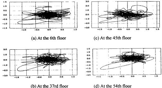
fig.11 acceleration track at different elevations (A<sub>max</sub>=0.225g\*C<sub>a</sub>)
