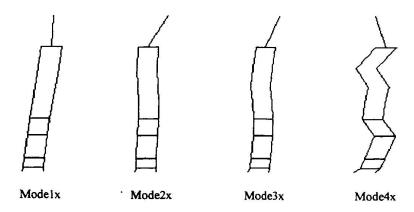
fig.8 Vibration mode shapes tested(X-Direction)
