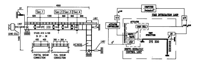
Fig. 1 Lay-out of substructure with full shear connection and relevant measurement apparatus
