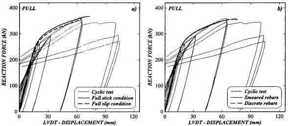
Fig. 6 Experimental and numerical results for full shear connection substructure:
