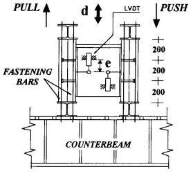
Fig. 8 Schematic lay-out of pull-push specimens
