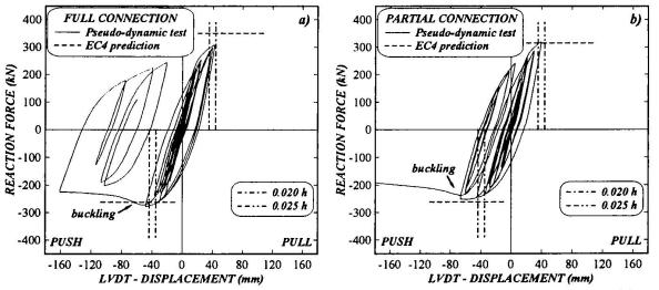
Fig. 4 Pseudodynamic hysteresis loops of reaction force vs. controlled displacement of substructure with:
