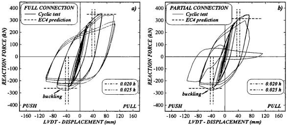
Fig. 3 Cyclic hysteresis loops of reaction force vs. controlled displacement of substructure with:
