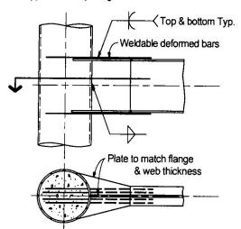
Type IV: Embedded Deformed Bar Connection
