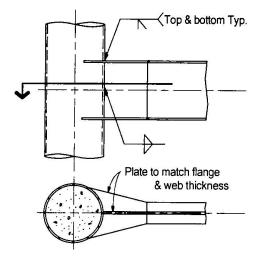
Type I: Simple Welded Connection
