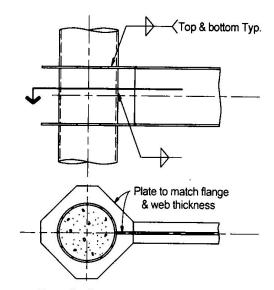
Type II: Diaphragm Plate Connection
