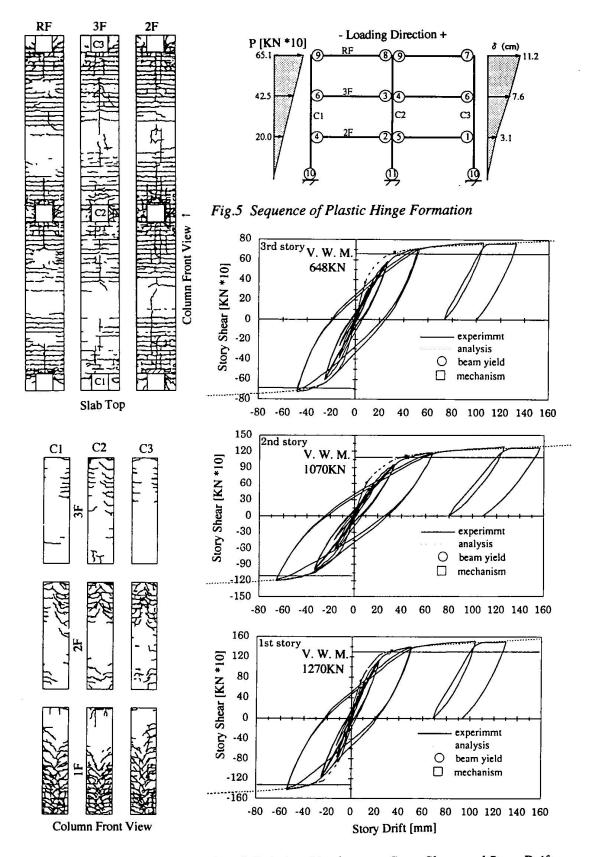
Fig.4 Observed Crack Patterns Fig.6 Relationships between Story Shear and Story Drift
