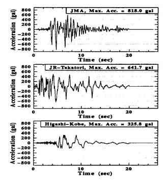
Fig. 4 Input Earthquake Accelerograms
