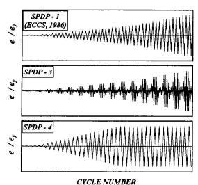
Fig. 9 Sequencial-phased displacement test procedures
