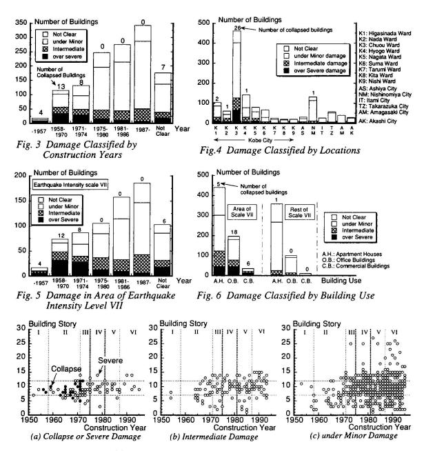
Fig. 7 Damage Classified by Story and Construction Year
