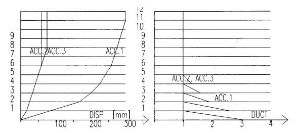
Fig. 8 Lateral displacements and column required ductility
