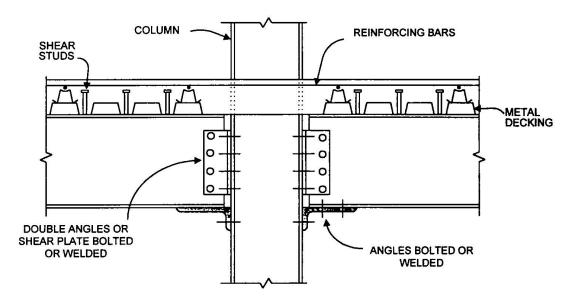
Figure 1 - Typical partially-restrained composite connection (PR-CC).
