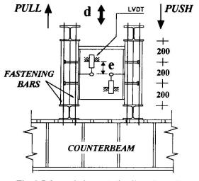
Fig. 8 Schematic lay-out of pull-push specimens
