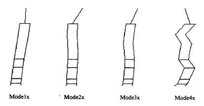
fig.8 Vibration mode shapes tested(X-Direction)
