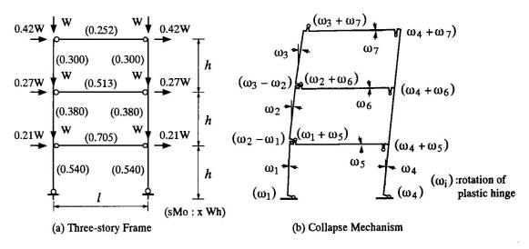
Fig.8 Three-story frame and the collapse mechanism
