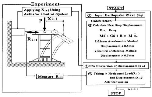
Fig. 3 A Flow Chart for Pseudodynamic Test Method
