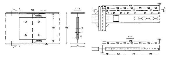
Fig. 3 The typical beam connection
