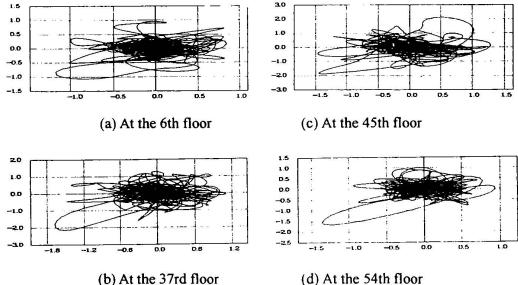
fig.11 acceleration track at different elevations (A<sub>max</sub>=0.225g\*C<sub>a</sub>)
