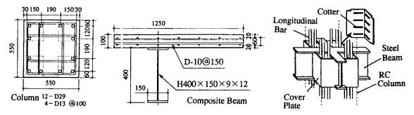
Fig.2 Column and Beam Section
