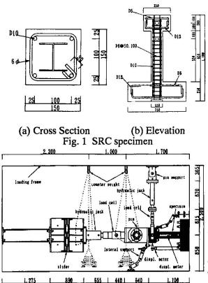
Fig. 2 Test set-up
