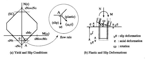
Fig,4 Yield and slip conditions and deformation mode
