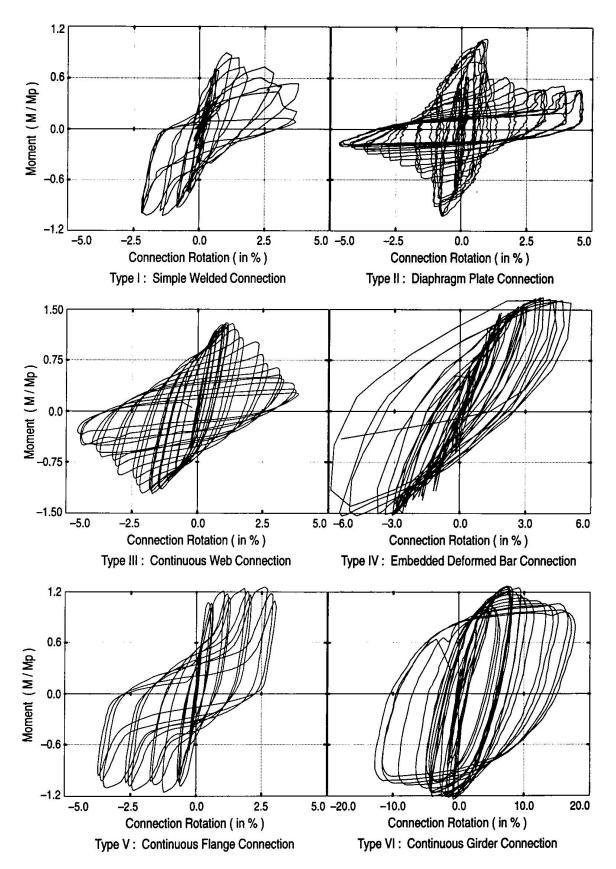
Figure 2. Experimental Moment-Rotation Behavior of Each Connection
