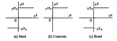
Fig.2 Stress-strain and bond stress-slip displacement relations
