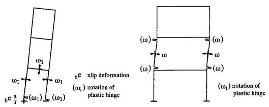
(a) Collapse Mechanism Considering Slip Deformation (b) Collapse Mechanism with Slab Diaphragm Effect
