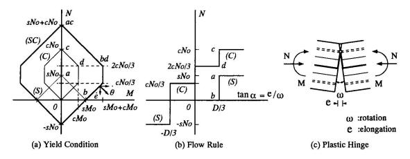
Fig.3 Yield condition and associated flow rule
