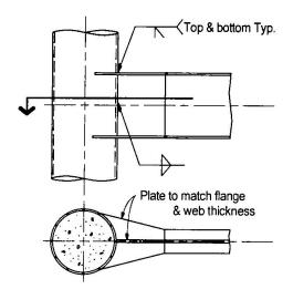
Type I: Simple Welded Connection
