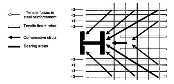
Figure 2 - Force transfer mechanism (simplified strut-and-tie model).
