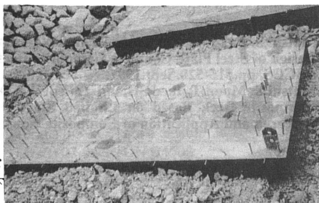
Photo.1 Typical shearing failure of studs
