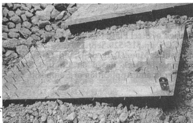
Photo.1 Typical shearing failure of studs
