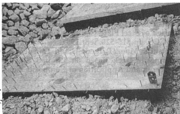
Photo.1 Typical shearing failure of studs
