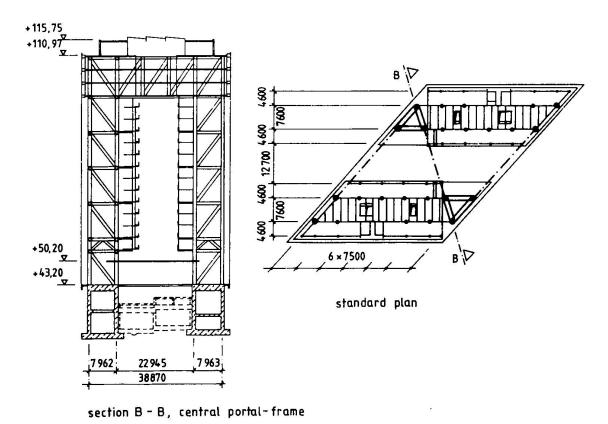
Fig. 8 Plan and section of the Towngate Düsseldorf
