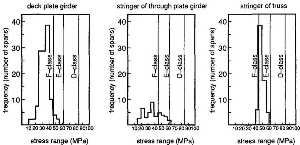
Fig.15 Variation of measured maximum stress range and fatigue assessments
