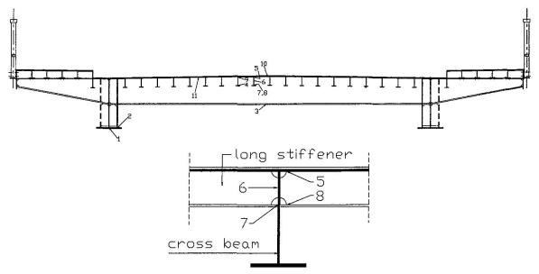
Fig. 6 Points considered for verifying fatigue resistance
