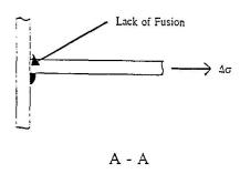
Figure 1: Fillet-welded connection of rib which is not continuous through the diaphragm
