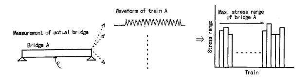
Fig.14 Maximum stress range of a bridge
