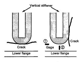
(a) Actual bridge (b) Fatigue test Fig. 7 Progress of crack
