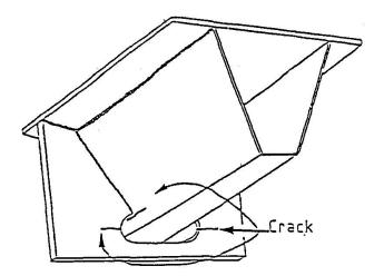
Figure 3: Diaphragm-to-rib connection showing typical crack locations at the cutout
