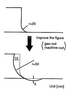
Fig.16 Improving work of flange gusset detail
