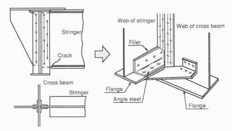
Fig.5 Damage of coped stringer
