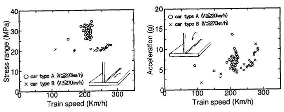
Fig.1 Relationship between train speed and stress range of flange or acceleration of web
