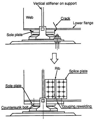
Fig.10 Damage of sole plate
