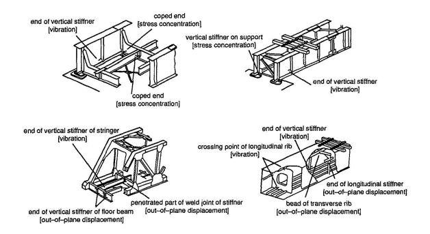
Fig.2 Fatigue damage in steel bridges
