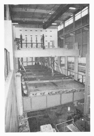
Figure 5 Full-scale fatigue test of a cantilevered section of an orthotropic deck.
