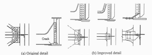
Fig.4 Improvement of details of cross beam
