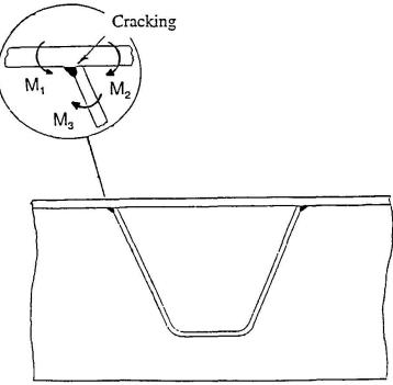
Figure 2: Distortion-induced cracking at longitudinal fillet-weld joining rib to deck plate
