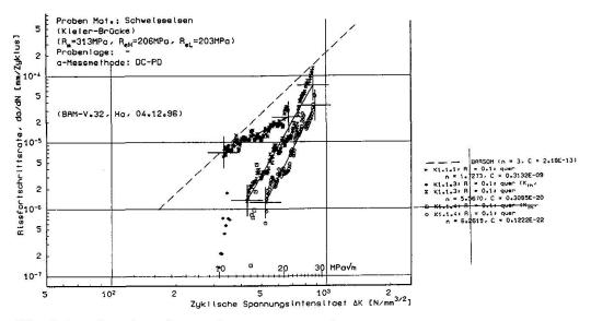
Fig. 2 Results of crack growth tests on wrought iron specimens
