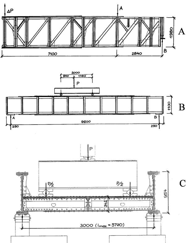
Fig. 1 Load arrangements: (A) main truss girder, (B) riveted plate cross girder, and (C) bridge parts made of wrought iron
