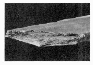
Fig. 7 Terrace crack in web plate
