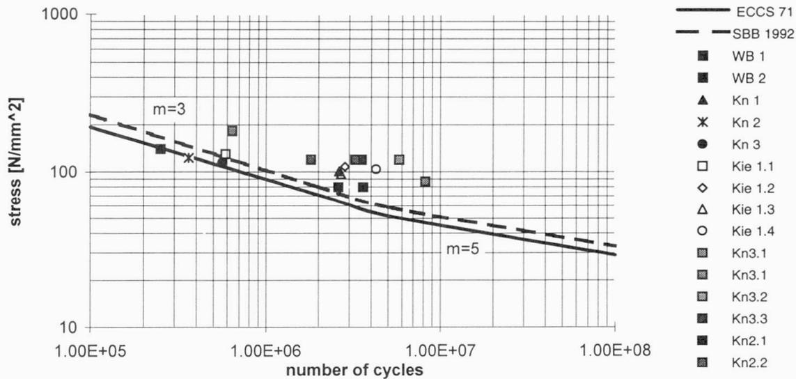
**Fig. 8** Results of full scale tests in S-N-curve
