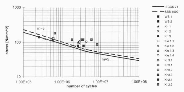
Fig. 8 Results of full scale tests in S-N-curve
