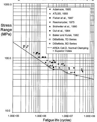
Fig. 6 Test Results + AREA, Normal Clamping, Superior Holes
