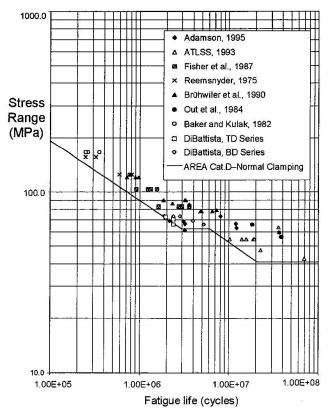
Fig. 5 Test Results + AREA, Normal Clamping
