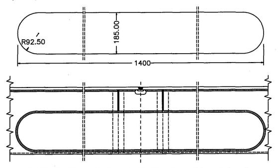
9— Fillet welding of the coverplates to the webs of the stiffener: the fillet side is equal to 6 mm. The fillet runs continuosly around the coverplate.
