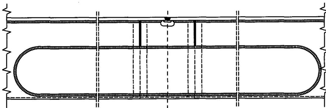
9- Fillet welding of the coverplates to the webs of the stiffener: the fillet side is equal to 6 mm. The fillet runs continuously around the coverplate.
