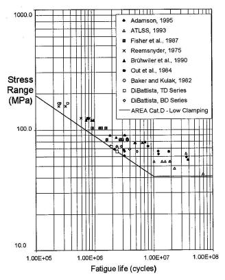
Fig. 4 Test Results + AREA, Low Clamping
