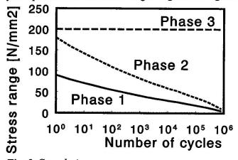
Fig. 2 Cumulative stress spectra
