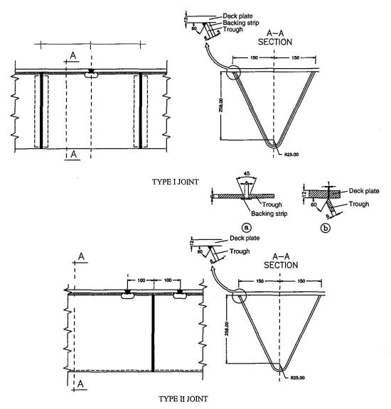
Fig. 1 Stiffener to stiffener connections
