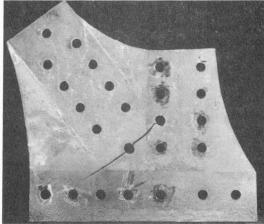
Fig. 3 Details of a cracked cover plate (A) concealed within the structure, (B) after disassembly
