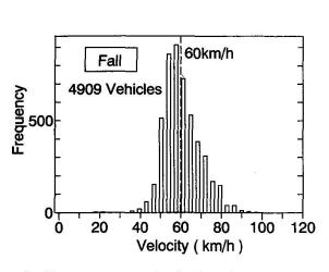
Fig.12 Frequency of vehicle velocity
