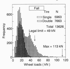
Fig. 10 Frequency of estimated wheel load
