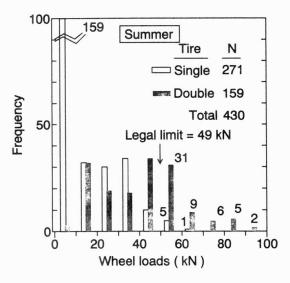
Fig. 7 Frequency of estimated wheel load position
