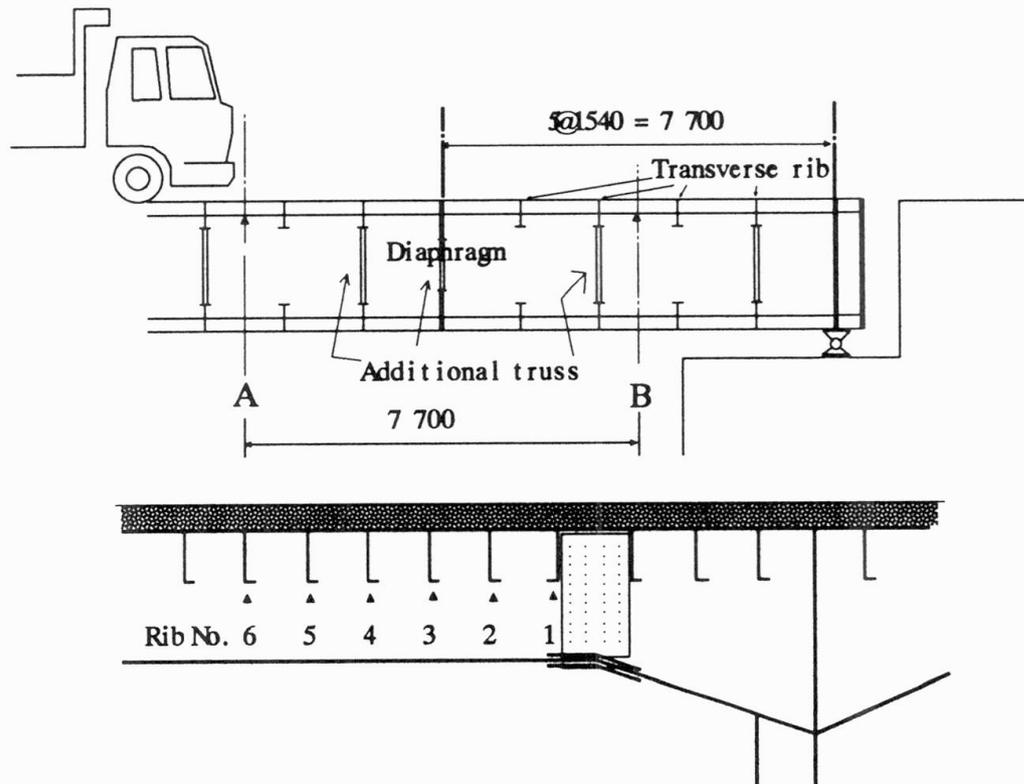
Fig. 2 Orthotropic steel deck of test bridge
