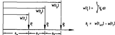
Determination of axle-distances at linear variable velocity  $v(t)$
