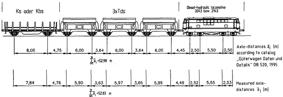
Fig.11 Checking of measured axle-distances for train 189
