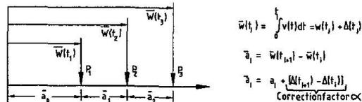
Fig. 10 Calculation of the corrected axle-distances  $\bar{a}_i$
