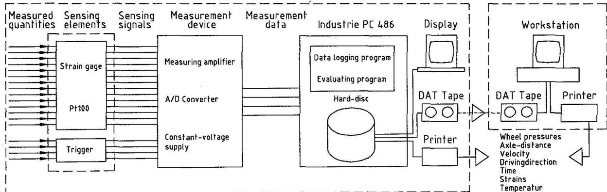
Fig. 4 Scheme of the measuring system
