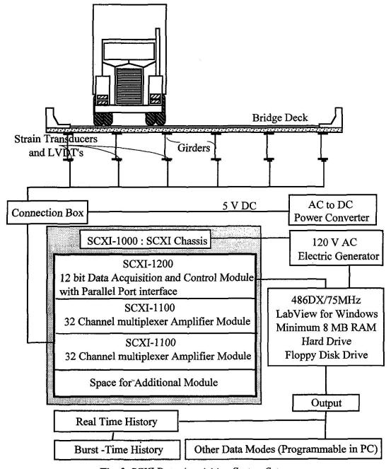
Fig. 3 SCXI Data Acquisition System Setup.
