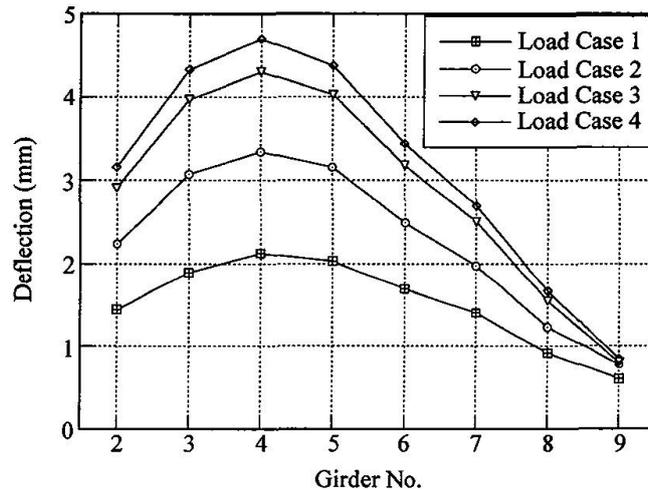
Fig. 9 Lateral distribution of deflections at mid-span for upstream loading
