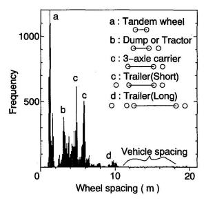
Fig.13 Frequency of estimated wheel spacing
