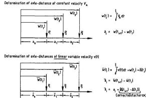
Fig. 10 Calculation of the corrected axle-distances  $\bar{a}_i$
