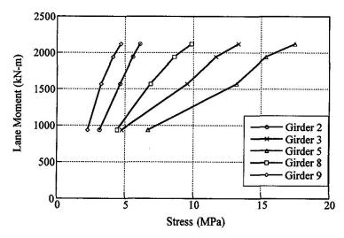
Fig. 5 Stresses at mid-span of girders for center loading
