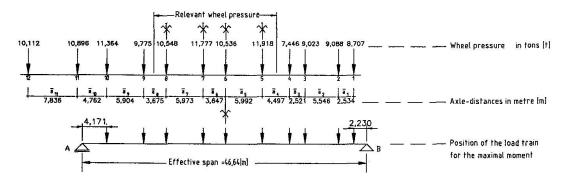
Fig. 12 The position of the train 189 for maximal bending moment in the middle of the bridge
