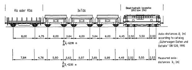
Fig. 11 Checking of measured axle-distances for train 189
