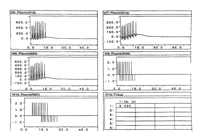
Fig. 6 Worksheet of strain-time histories and trigger-signals and velocity for the train 189 in the "measuring area a"
