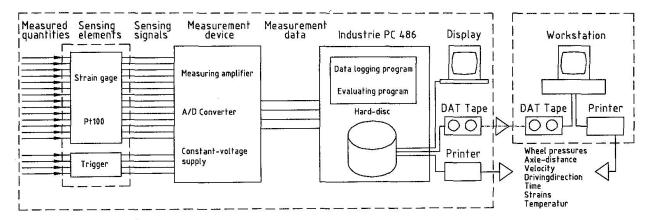
Fig. 4 Scheme of the measuring system
