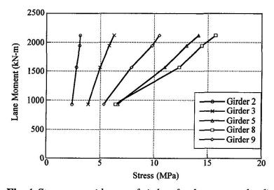
Fig. 4 Stresses at mid-span of girders for downstream loading
