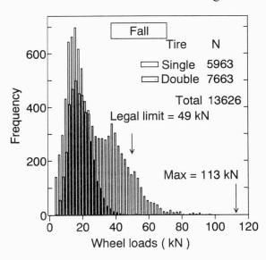
Fig. 10 Frequency of estimated wheel load
