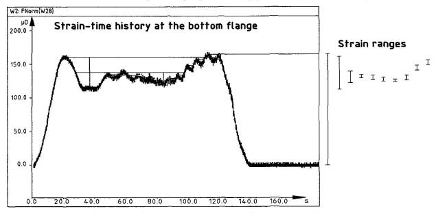
Fig. 13 Strain-time history in the measuring point at the bottom flange during the running of the train 278.
