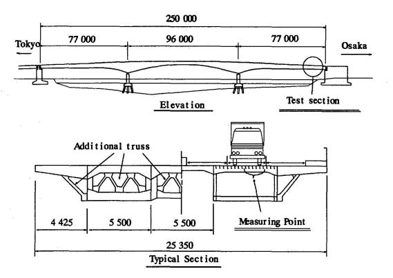
Fig. 1 Orthotropic steel deck bridge
