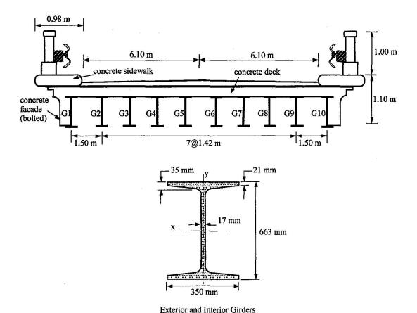
Fig. 1 Cross-section of the tested bridge
