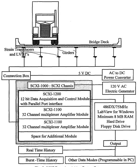
Fig. 3 SCXI Data Acquisition System Setup.
