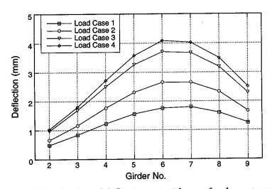
Fig. 7 Lateral distribution of deflections at mid-span for downstream loading
