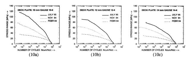
Fig. 10 Measured stress spectra stiffener deck plate connection - 60mm mastic asphalt surfacing
