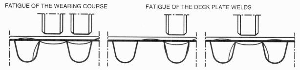
Fig. 1 Effects of local wheel loading on orthotropic steel bridge decks
