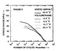
Fig. 15 Measured stress spectra Caland bridge 10 mm deck plate and 50 mm surfacing
