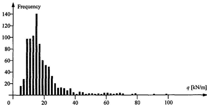
*Fig. 4 Histogram of measured heavy-vehicle linear-weight,  $q$*
