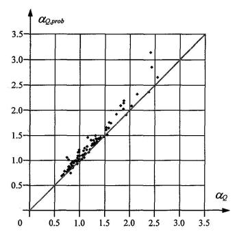
Fig. 3 Comparison of traffic action effect reduction factors derived using the probabilistic approach,  $\alpha_{O,prob}$ , and the simple method,  $\alpha_{O}$ .
