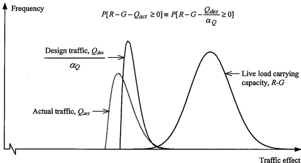
Fig. 1 Calibration of traffic action effect reduction factors
