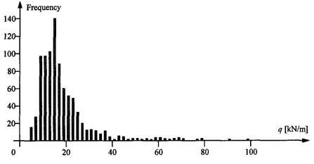
Fig. 4 Histogram of measured heavy-vehicle linear-weight, q
