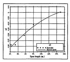
Fig. 5 Plot of real values of al and a2 and best fit curve for the case of continuous bridges and heavy traffic conditions
