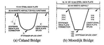
Fig. 9 Strain gauge locations
