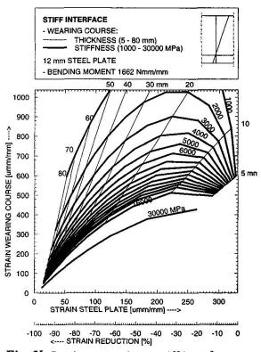
Fig. 3b Strains assuming a stiff interface.
