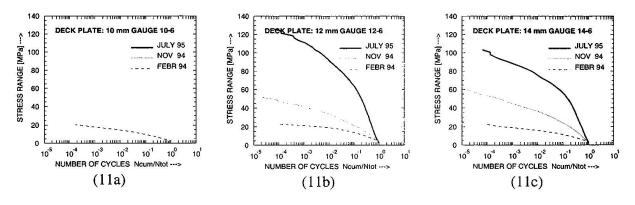
Fig. 11 Measured stress spectra longitudinal deck plate splice - 60 mm mastic asphalt surfacing
