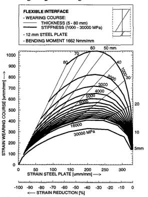
Fig. 3a Strains assuming a flexible interface.
