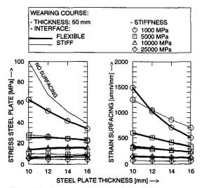
Fig. 4 Influence of steel plate thickness
