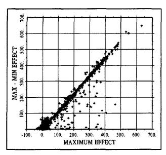
Fig. 2 Plot of increments of effect vs maximum effect for a simply supported (left) and a continuous (right) bridges
