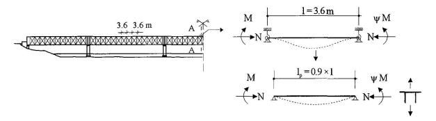
Fig.4 Simplified structural model for reliability analysis
