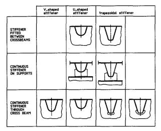
The introduction of the closed V-shaped, U-shaped and trapezoidal stiffeners as shown in Fig. 2, was a large improvement, which alloyed spans of approximately 4.0m. The secondary crossbeams and main girders were no longer needed. The amount of work involved reduced as well as the costs.
