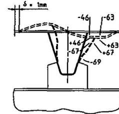
It is obvious that these stresses which mainly are governed by bending effects in the deck plate and trough web, can not be neglected. The stress concentration factors related to the bottom connection are assumed to be higher than the stress concentration factors related to the trough to deck connection. If however the stresses due to the wheel loading on the deck are added, high stress amplitudes may occur due to the combination of both effects.
