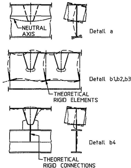
**Fig. 6** Closed stiffener connections and structural behaviour
