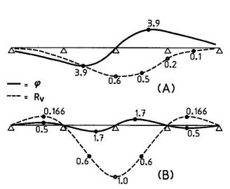
**Fig. 15** Influence lines for stiffener support rotations (f) and reactions  $(R_v)$
