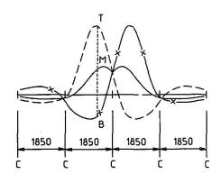
Fig. 16 Influence line stresses outer side web plate location "P"
