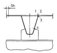
Fig. 18 Relevant locations for fatigue
