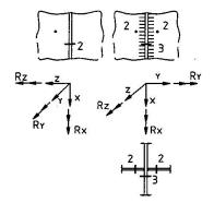
Fig. 13 Fatigue locations and degrees of freedom detail "a"
