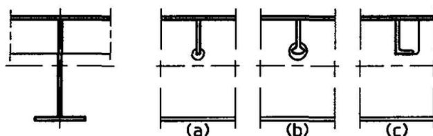
Fig. 5 Crossbeam connections with continuous open stiffeners
