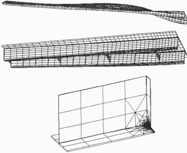
Fig 3 Finite elements modelling of the joint
