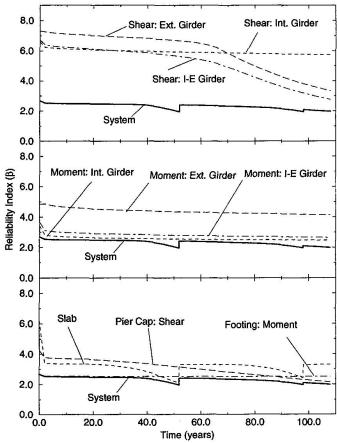
Fig. 6 Updated results of repair option 1 on Bridge E-17-AH using simplified series-parallel model requiring the failure of three adjacent girders
