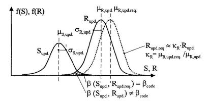
Fig. 5 Calibration of updated load and resistance models
