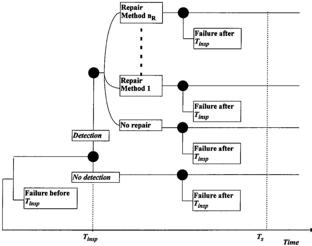
Fig.2 Events tree for a conditional maintenance model
