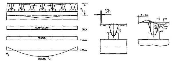
Fig. 9 Model of floating deck crossbeam
