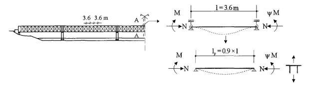
Fig.4 Simplified structural model for reliability analysis
