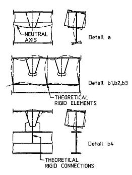
Fig. 6 Closed stiffener connections and structural behaviour
