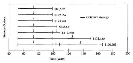
Fig. 7 Updated strategy options and costs (2% discount rate) for Bridge E-17-AH using simplified series-parallel model requiring the failure of three adjacent girders
