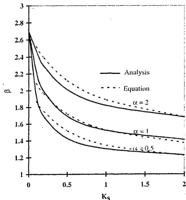
Fig. 7.  $\beta$  factors vs  $K_s \leq 2$  for selected values of  $\alpha$  in sub-frame F3.
