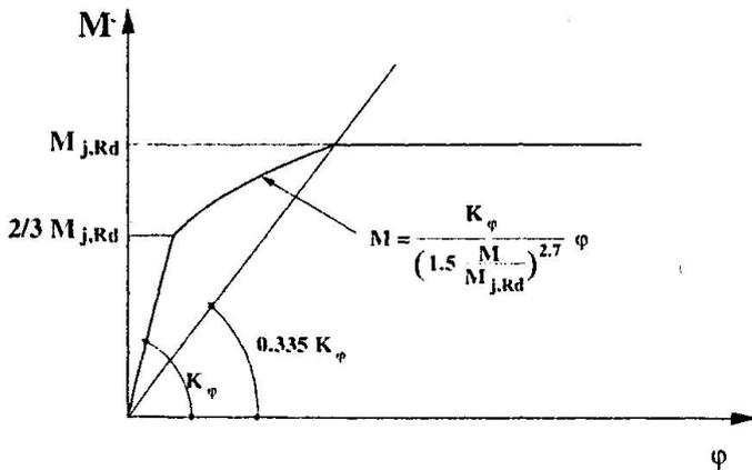
Fig.4 - Moment-rotation curve according to Annex J
