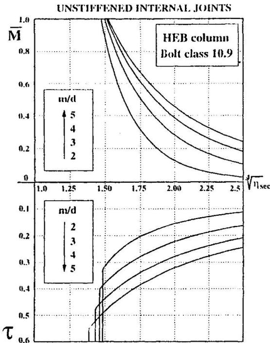
Fig.5 - Design abacus for unstiffened internal joints
