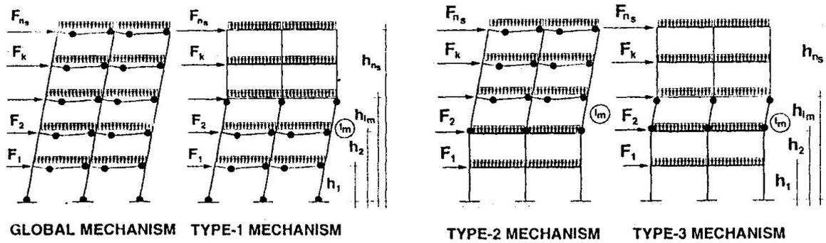
Fig.1 - Analysed collapse mechanism typologies
