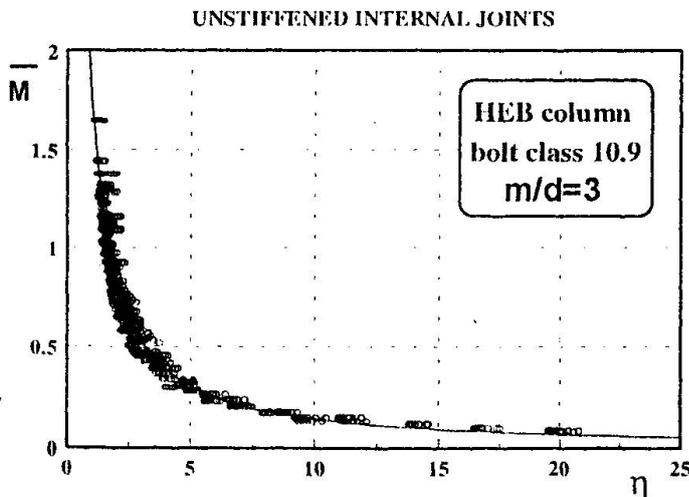
Fig.2 -  $\bar{M} - \eta$  relationship for unstiffened internal joints and  $m/d=3$
