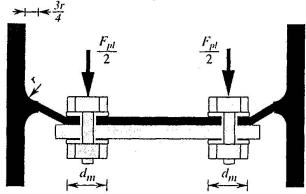
Fig. 6. Failure mechanism of bolted connection
