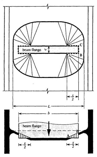
Fig. 9. Combined flexural and punching shear failure
