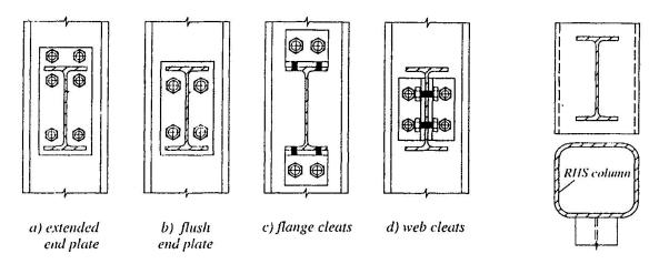
Fig. 1. Beam-to-I section column minor-axis joints
