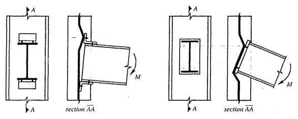
Fig. 3. Local mechanism
