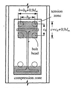
Fig. 8. Bolted connection
