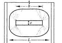
Fig. 5. Yield line pattern (Local mechanism)
