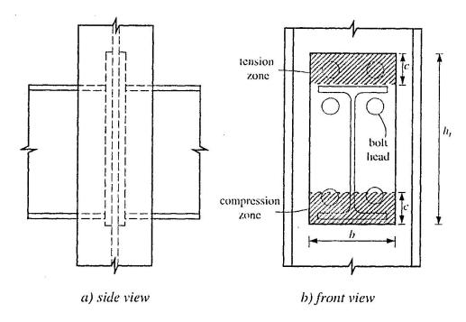
Fig. 13. Joint with two beams one of each side of the column web
