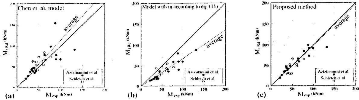
Fig.4 - Reliability of different procedures for predicting the flexural resistance
