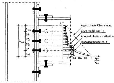
Fig. 3 - Plastic shear of the web angle
