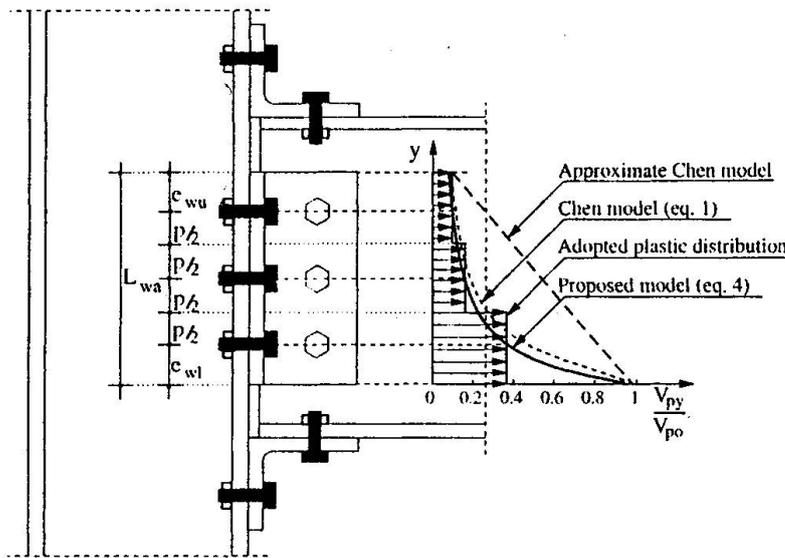
Fig. 3 - Plastic shear of the web angle
