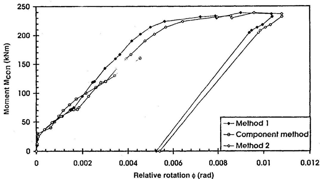
Fig. 5. Moment-rotation data obtained using three different methods.
