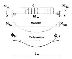
Fig.1. Scheme for beam line
