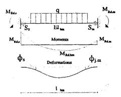
Fig. 6. Scheme for a beam in sub frame
