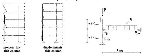
Fig. 4. Moments and displacements of the Fig. 5. Scheme of the analytical model outer column
