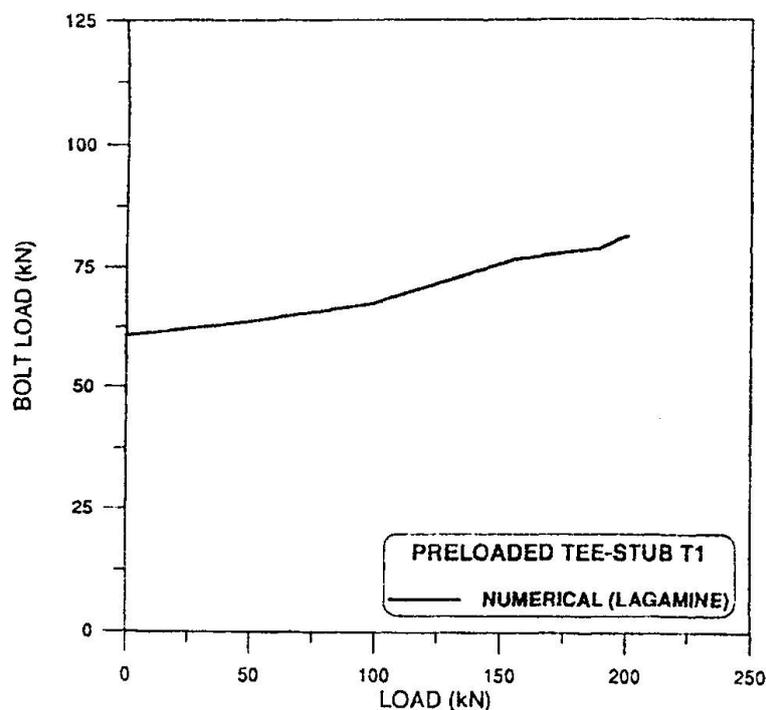
Fig. 7 Bolt axial force versus total force  $F$  for the preloaded tee-stub T1
