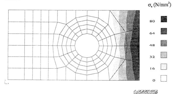
Fig. 5 Normal pressure distribution at the failure state for the preloaded tee-stub T1
