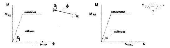
Fig. 2. M-\phi diagram of a joint
