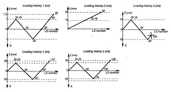
Figure 4. The loading sequence for the loading cases considered
