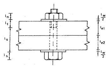
Fig. 2 Bolt geometry
