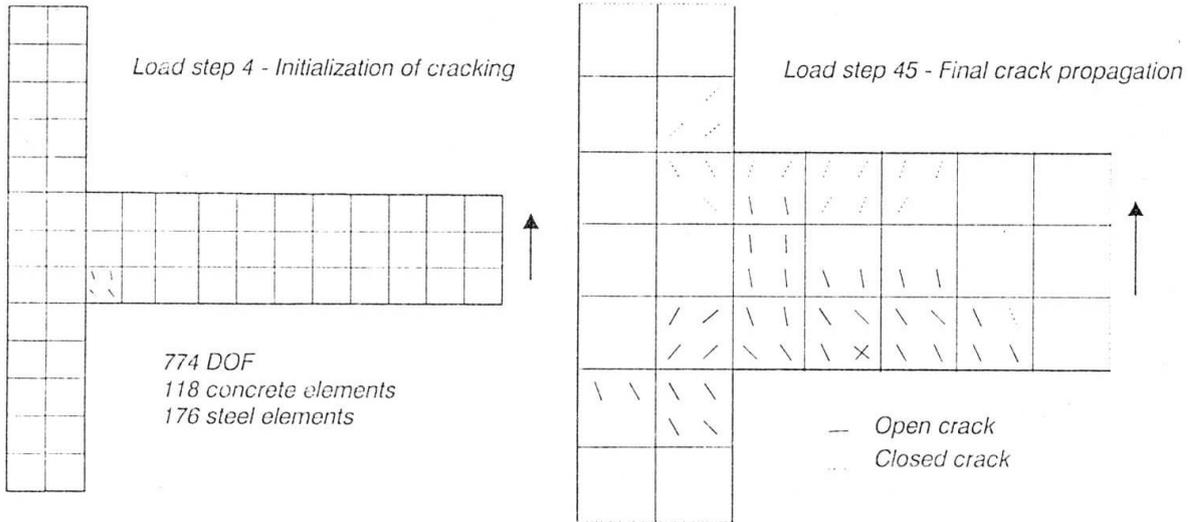
Figure 5. Loading case 1 - FE mesh data and tensile crack development at load step 4 (0.4 mm) and load step 45 (1.5mm)
