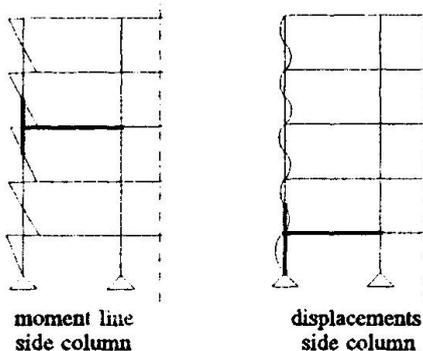
Fig. 4. Moments and displacements of the outer column
