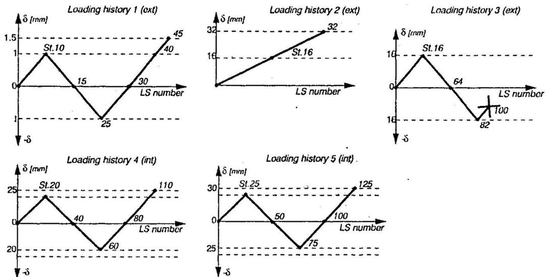
Figure 4. The loading sequence for the loading cases considered
