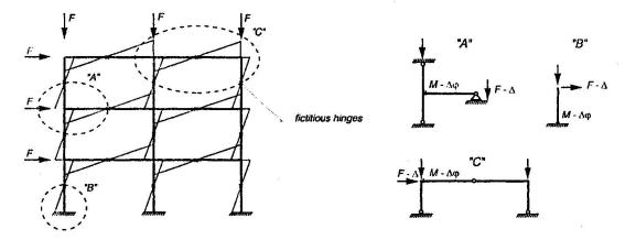
Figure 1. The bending moment diagram of a plane frame, loaded laterally and the identified substractures
