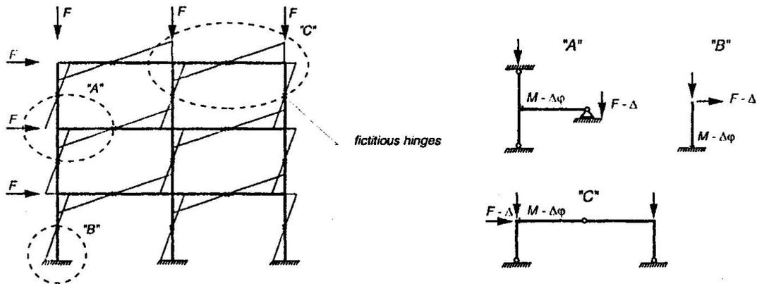
Figure 1. The bending moment diagram of a plane frame, loaded laterally and the identified substructures
