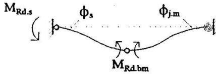
Fig. 9. Last hinge in mid joint
