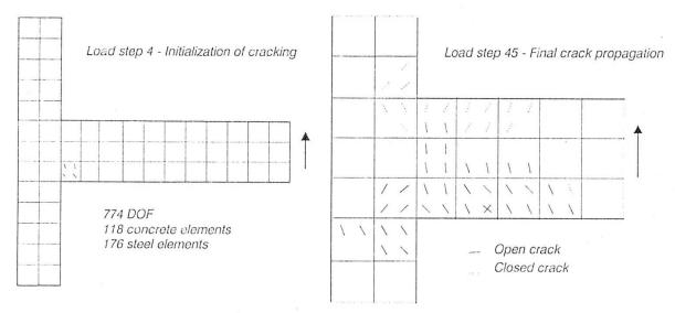
Figure 5. Loading case 1 - FE mesh data and tensile crack development at load step 4 (0.4 mm) and load step 45 (1.5mm)
