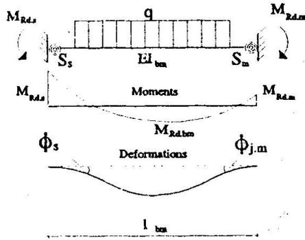
Fig. 6. Scheme for a beam in sub frame
