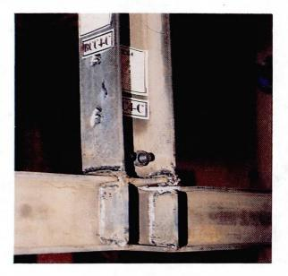
Fig. 4. Experimental moment-rotation diagram and failure mode of BCC4 connection type.
