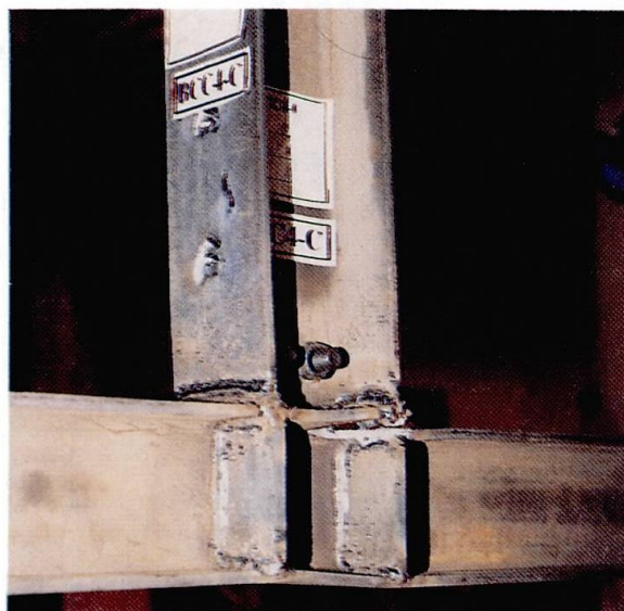
Fig. 4. Experimental moment-rotation diagram and failure mode of BCC4 connection type.
