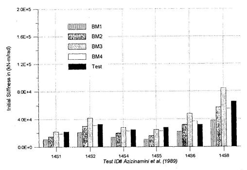
Figure 4. Finite Element and Test Results for Top and Seat with Double Web Angle Connections.
