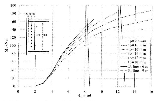
Fig. 6. "Moment--rotation" curves of single web plate joint.
