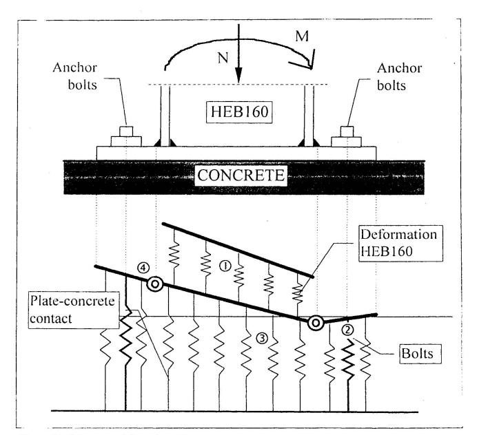
Fig. 4. Modelisation of the column bases connections
