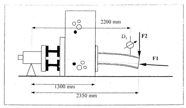
Fig. 2. Determination of the joint bending moment.
