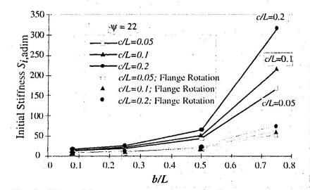
Fig. 6 - Effect of flanges rotation on initial stiffness
