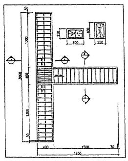
Figure 1. Details of Ductile Specimen
