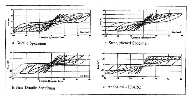
Figure 10. Load-Displacement Curves
