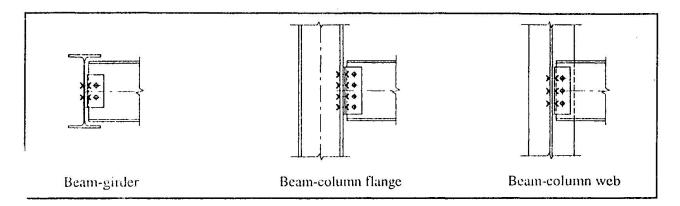
Fig. 2. Three typical double web cleat connections.
