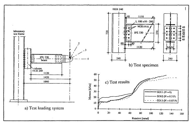
Fig. 4. Bare steel connection tests.
