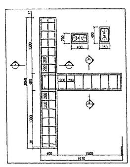
Figure 2. Details of Non-Ductile Specimen
