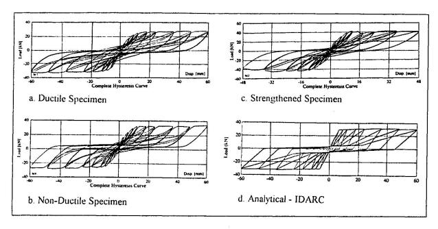
Figure 10. Load-Displacement Curves
