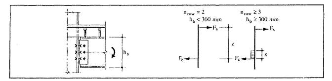
Fig. 7. Simplified model for composite joints with double web cleat connections.
