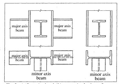
Fig. 3 - (a)Restrained and (b)unrestrained column flanges.
