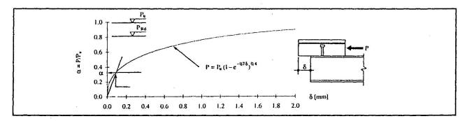
Fig. 8. Load-slip behaviour of a shear stud connector ([9]).
