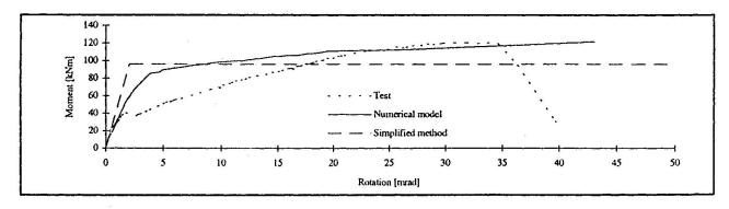
Fig. 9. Comparison between the test result, the numerical model and the simplified method.
