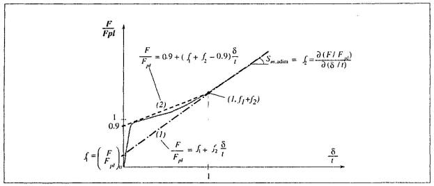
Fig. 8 - Bi-linear approximation of column web post-limit behaviour
