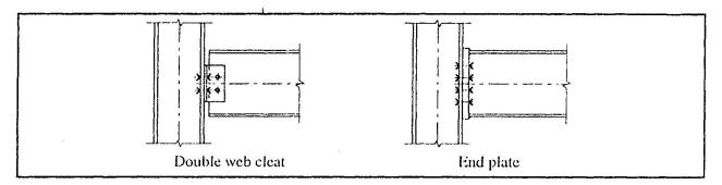
Fig. 1. Typical steel beam-to-column joints.
