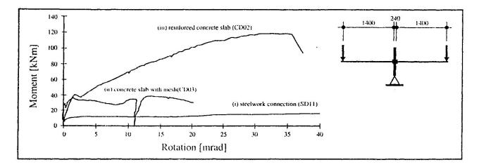
Fig. 6 Moment-rotation curves for composite joint tests.
