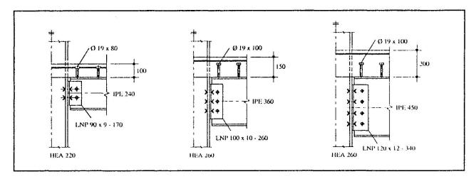
Fig. 3. Typical detailing of composite joints with double web cleat connections.
