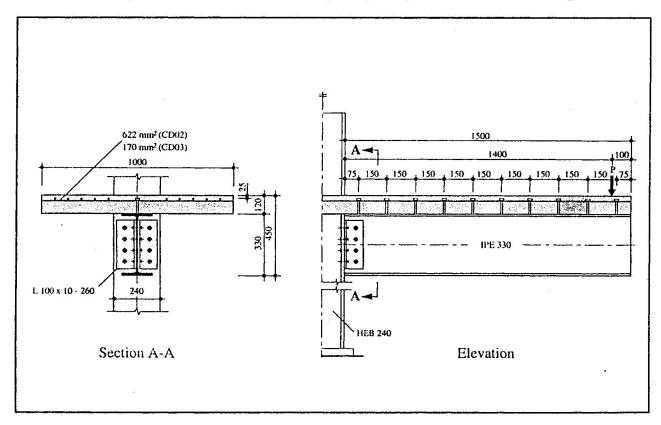
Fig. 5. Composite joint specimen.
