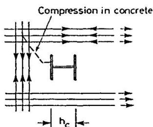
Fig. 8. Out-of-balance loading
