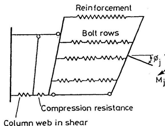
Fig. 10. EC3 mechanical model
