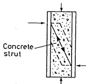
Fig. 7. Encased column web in shear
